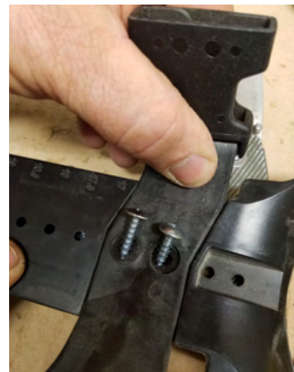
6A. Replace with new Strap Mount screws. (Note 2 different size screws and placement).
