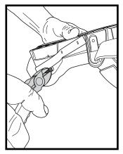
3. Remove Cushion Insert by carefully clipping both Cable Ties that secure the Cushion to the frame.
