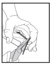
10. Tighten Cable Tie with pliers.
