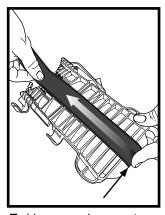
5. Line up replacement Hook 'n Loop and stick to the bottom front of the frame.
