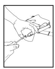
**12.** Replace all 6 screws securing the boot to the frame.
