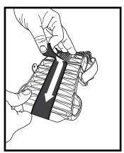
**4.** Remove old 1½" x 10 ¾" Hook 'n Loop from frame. (Leave all stapled 1/2" Hook 'n Loop in place)
