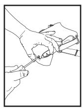
1. Remove all 6 screws securing the boot to the frame.
