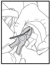
**11.** Carefully clip off excess Cable Tie and and Install new 1" liner. Refer to "Replacing the AP16 No Wrinkle Liner" on back, if needed.
