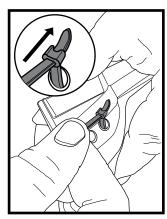
9. Thread through Cable Tie end and pull.
