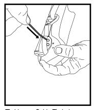
**7.** Line up Cable Tie holes on frame and Cushion. Thread Cable Tie through the left hole and up through the Cushion Insert.
